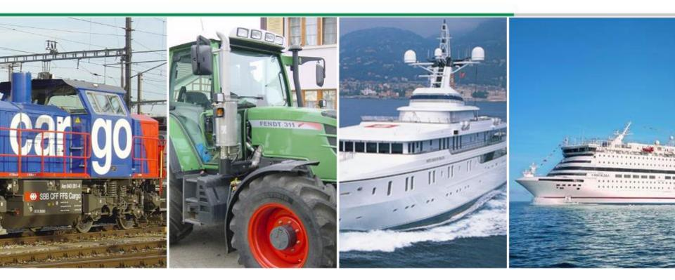
200 – 5,000 kW (270 – 7,000 HP) Soot filter, SCR, Oxi 15 - 650 kW (20 – 900 HP) Soot filter, SCR, Oxi 200 – 5,000 kW (270 – 7,000HP) Soot filter, SCR, Oxi 1,000 – 40,000 kW (1,350 – 54,000HP) Soot filter, SCR, Oxi
