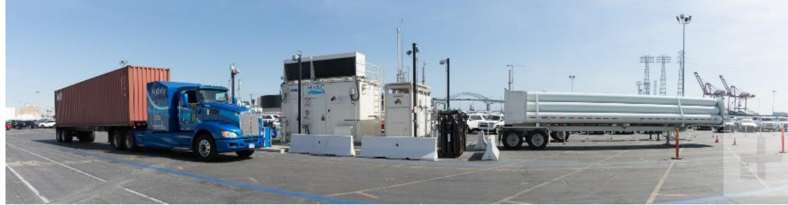
Fuel Cell Electric Kenworth Model T680 developed in collaboration with Toyota refueling at Toyota's Port of Long Beach Terminal
