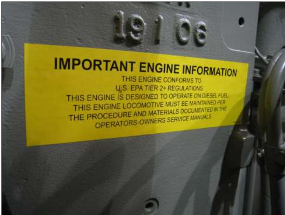
A supplemental label on an engine.
