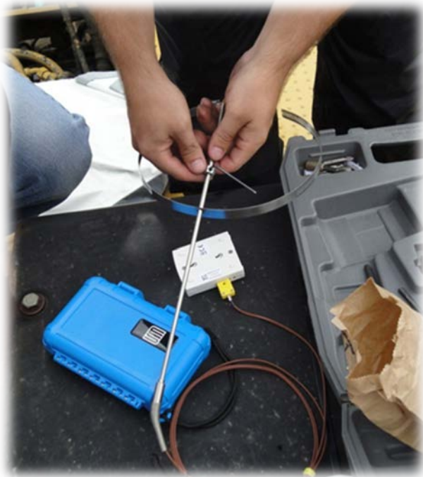
Thermocouple probe, mounting clamp, data logger, and protective housing
