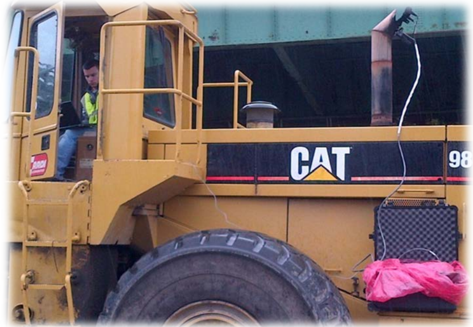
Opacity metering in progress
