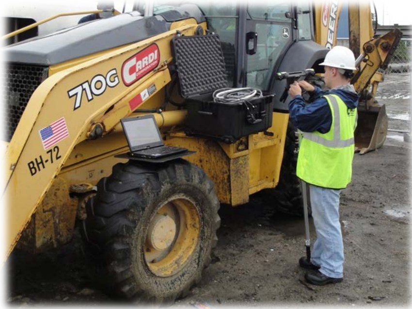
Preparing for testing – laptop, opacity meter, sensor head
