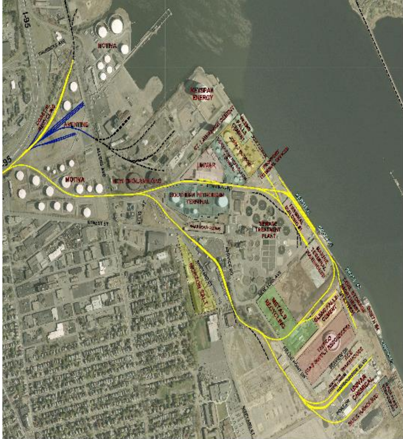
South Providence and Port of Providence. The blue lines indicate the new track consisting of the South Providence yard and the ethanol unloading facility [see photo in 07#03B], owned by Motiva through which Aventine ethanol will flow. Yellow lines show the track, operated by PW, leading into ProvPort. (map courtesy Joshua Moldover)
